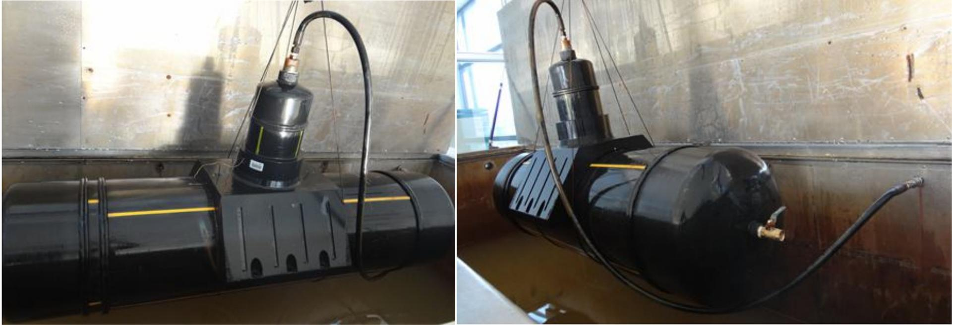
Smart Joint conduct all necessary tests required by ISO standard for the produced Electrofusion Saddle. All tests pass.
